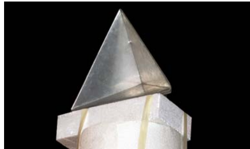
Figure 14: Corner Reflector on Polystyrene Column
